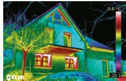
Thermal imaging cameras are an excellent tool to verify whether insulation repairs are effective.
