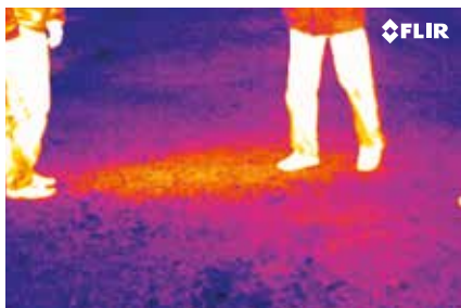
With a thermal imaging camera the exact location of the leak is easily spotted.
