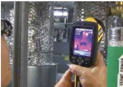
FLIR thermal imaging cameras can be used to detect a multitude of different heat related building issues.
