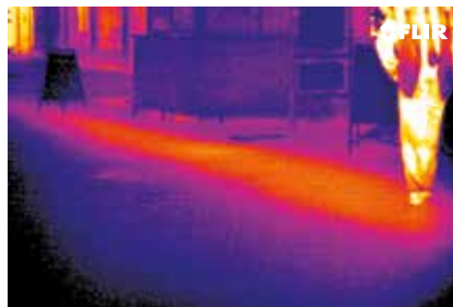
Thermal imaging cameras make the underground pipes of a district heating network clearly visible. Leaks in the network can easily be spotted
