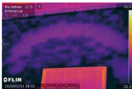
This thermal image shows that below the surface this wall contains arches for better weight distribution.
